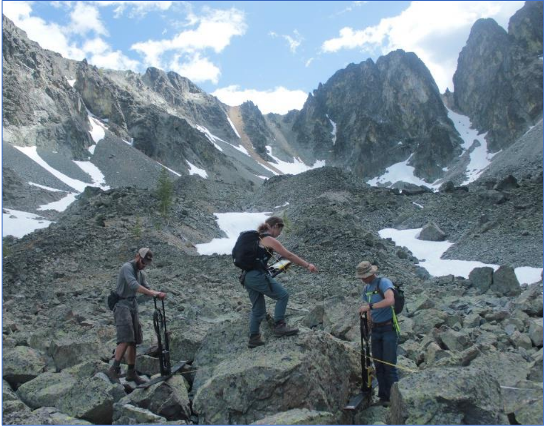
Figure 4.3. The PulseEKKO PRO GPR survey at the Eightmile Creek 1 rock glacier. This image shows the transmitter (left), the DVL (center), and the receiver (right) during a transverse survey across the unstable terrain typical of rock glacier surfaces. Photo captured by Bailey Duvall, 7/13/2020.
