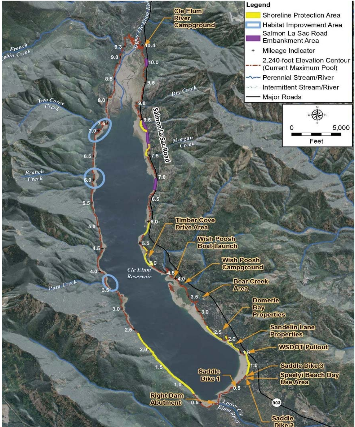
Figure 42: Cle Elum Lake reservoir expansion shoreline protection. Includes rockery walls, anchored logs, and perched beaches (BOR and WADOE 2015).
