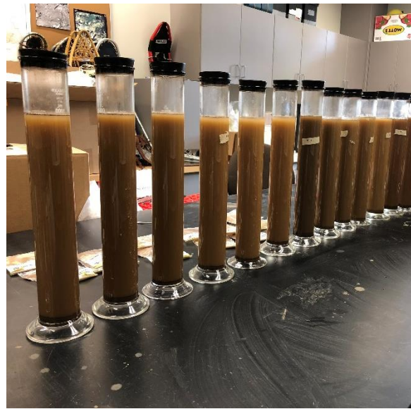
Figure 13. 1000ml graduated cylinder after agitation. Image from Ellie Myers, 2018.
