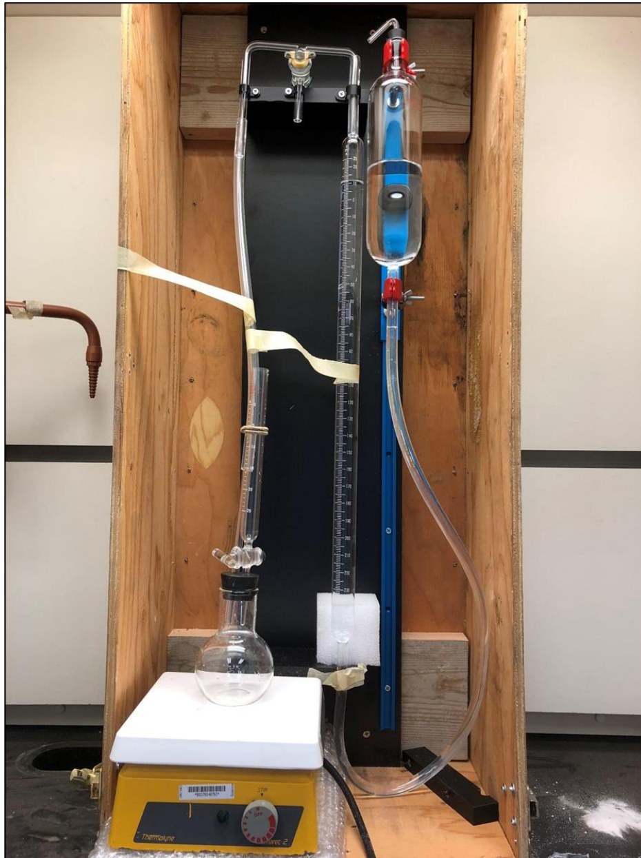
Figure 17. Chittick Apparatus. Image from Ellie Myers, 2018.
