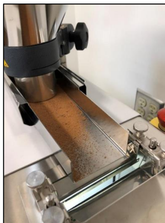
Figure 16. Camsizer P4 vibrating chute. Image from Ellie Myers, 2018.
