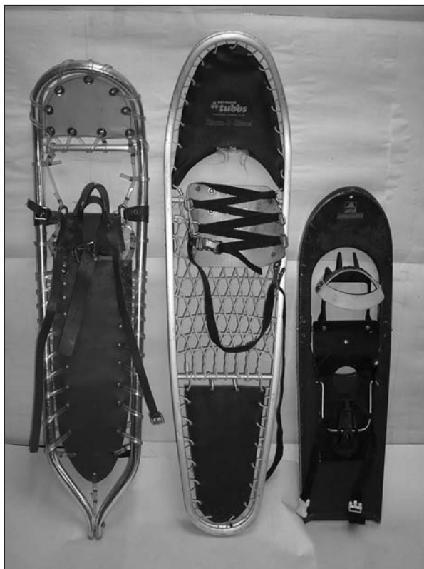
Figure 5.—Late 1970s and 1980s Prater “Ellensburg” (left), Tubbs “Alum-A-Shoe” (middle), Polar Equipment Company’s “Polarpaws” (right). Note the Westover-modified frame on the Praters, the aluminum I-beam frame, Hypalon decking, and plastic-coated wire lacing on the Tubbs, and integrated sheet-aluminum frame-decking-traction of the Polarpaws.
