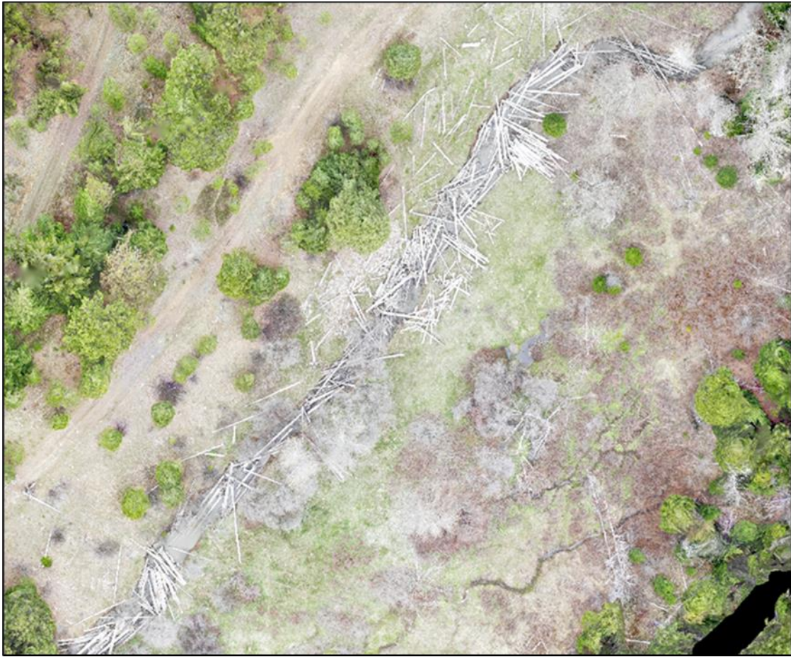
Figure 4. Aerial photo of instream large wood restoration of Indian Creek near North Fork Teanaway road just upstream from the DOE gauge (Figure 5A). (Image credit: Isaac Mitchell)
