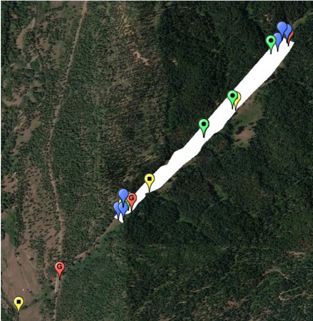
Figure 25. Area polygon used for potential storage capacity. The polygon extends from the furthest upstream well to the furthest downstream well; from the approximate location of the stream channel to the northern hillside.
