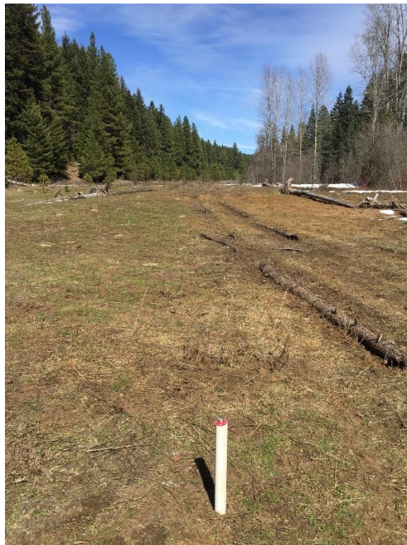
Photo D- 8: Piezometer installed by Nora Boylan in October 2018.
