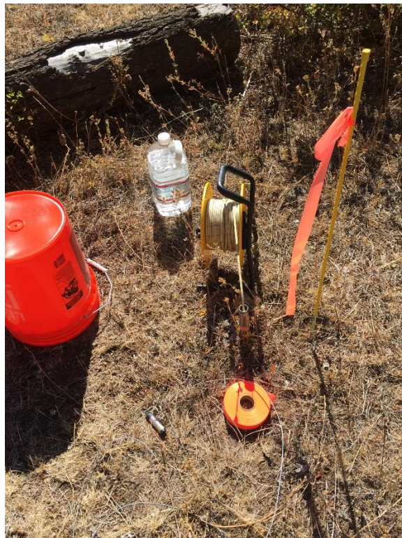
Photo D- 6: Example of slug test setup at MP-2. Photo taken in October 2018.
