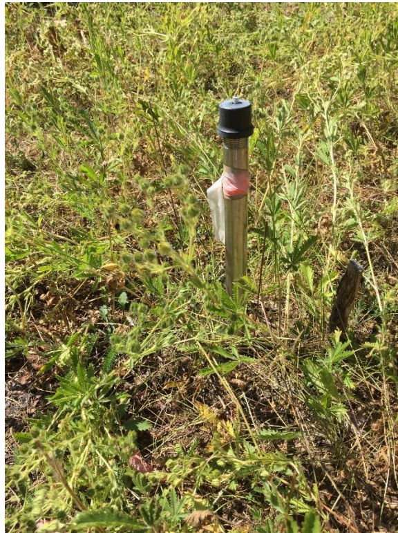
Photo D- 4: Piezometer installed in 2014 by Ecology, WDFW and KCT. Photo taken in June 2018.
