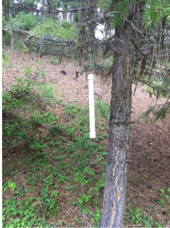
Photo D- 11: PVC pipe holding barometer used for water level compensation. Photo taken in June 2019.
