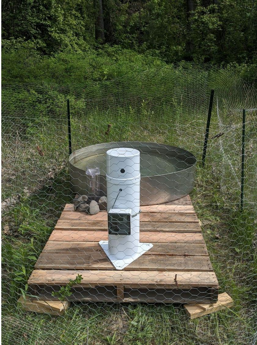
**Figure 48.** Evaporation pan and precipitation gauge. This equipment was installed at the riparian site. The tall white cylinder is the evaporation gauge, which is directly connected to the pan and records its water level. The precipitation gauge is next to the pan (transparent, surrounded by rocks).
