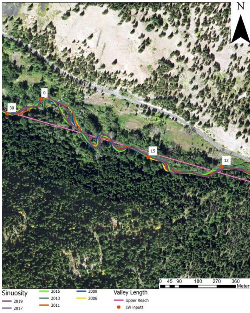
Figure 15: An example of the sinuosity measurements at the upper reach. The numbers next to the LW inputs are the number of LW pieces. The straight pink line represents the valley length.
