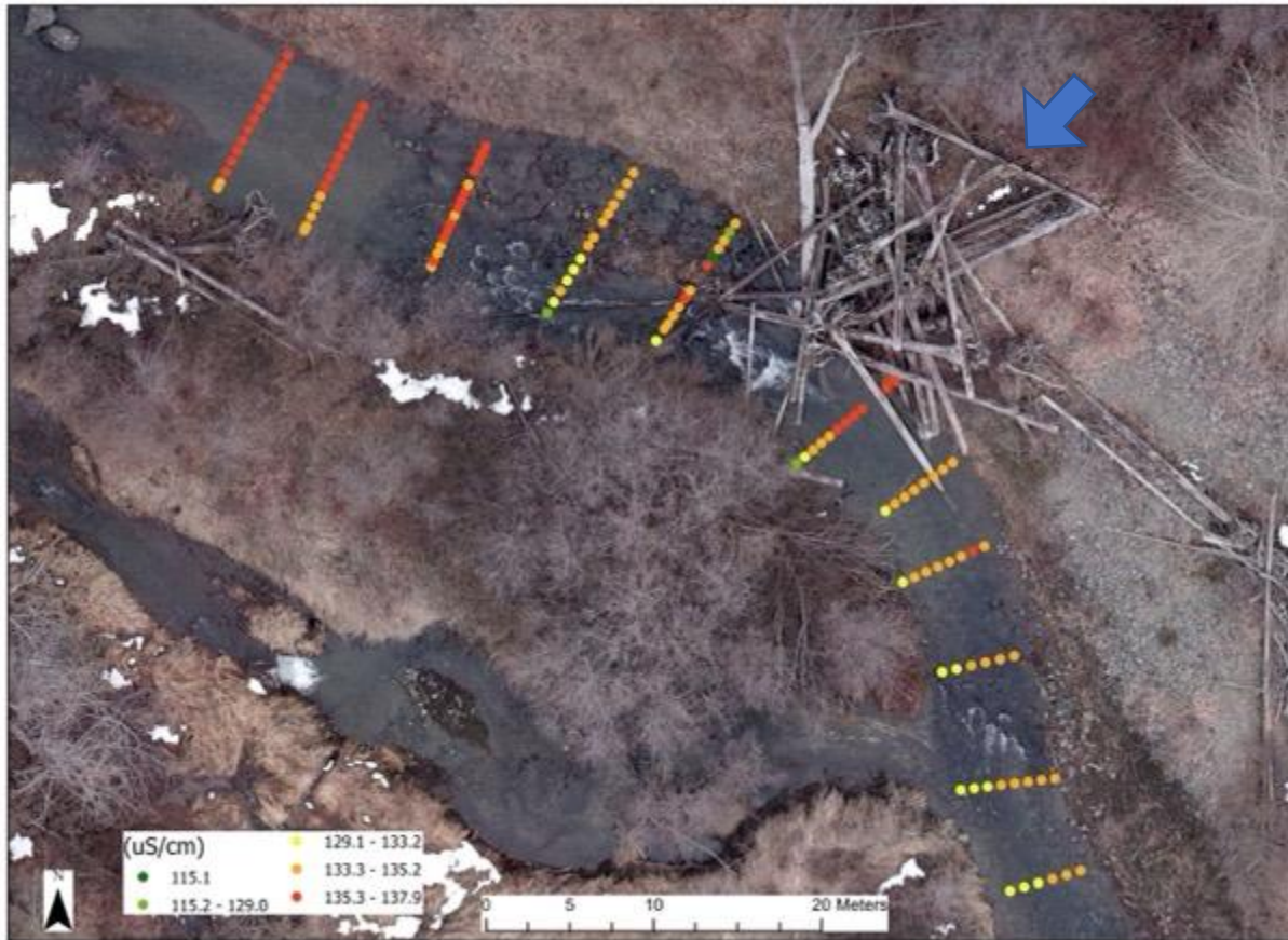
Figure 22: The salinity values \mu\text{S}/\text{cm} for the Middle Reach LW reach. The salinity values were higher on the immediately downstream of the LW and on the left bank. The blue arrow indicates the location of the LW jam.
