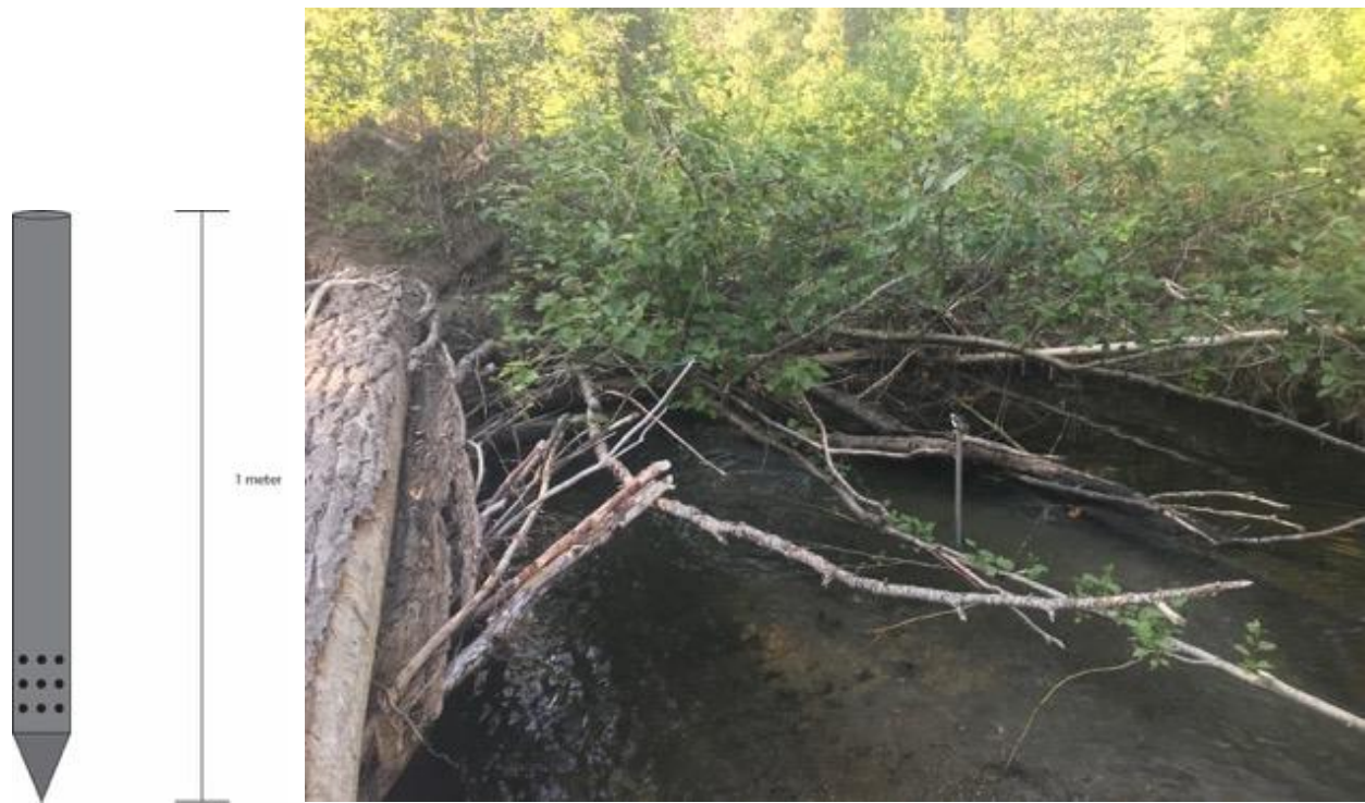
Figure 11: Left- The piezometer, which is 1m in length. The slotted ends were driven into the bed substrate as far as possible. Right- The piezometer at the middle reach, downstream of a LW log jam.
