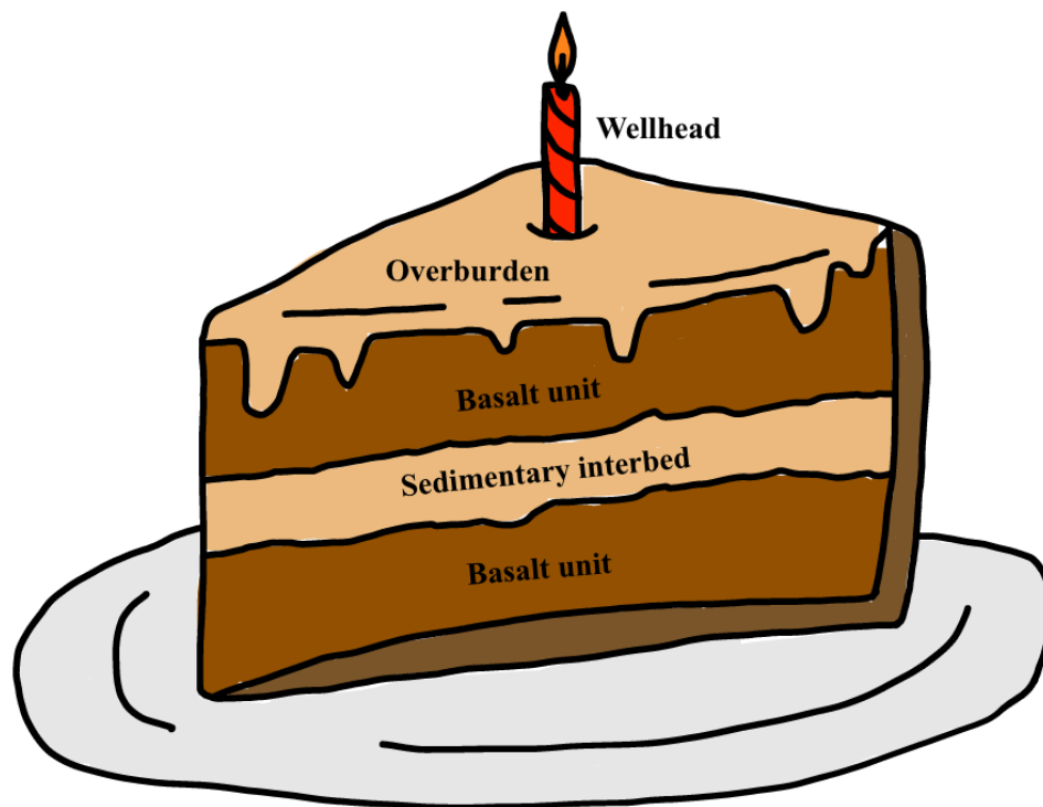
Figure 8. Illustration of the stratigraphic “layered cake” sequence of basalt units as cake and interbedded sediments as filling between them. The icing represents the overburden, and the candle symbolizes a well that penetrates the subsurface.
