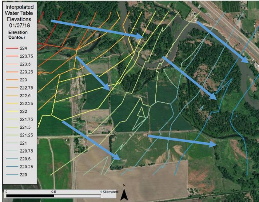
Figure 42. Water elevation contour lines interpolated from water level elevations using Empirical Bayesian Kriging in ArcMap 10.5. Blue lines indicate general direction of groundwater flow on 01/07/2018.
