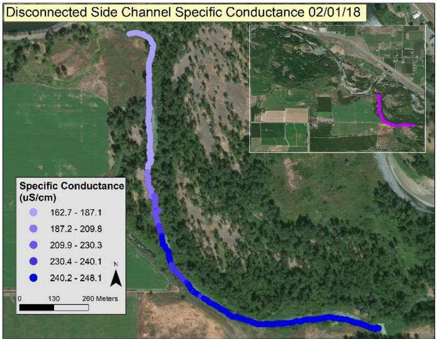
Figure 28. Specific conductance of disconnected side-channel in winter.
