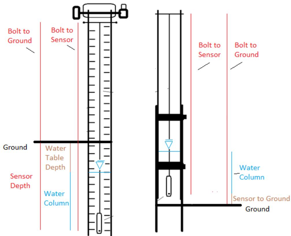
Figure 12. Measurements used to calculate water level elevations from digital elevation model raster values.
