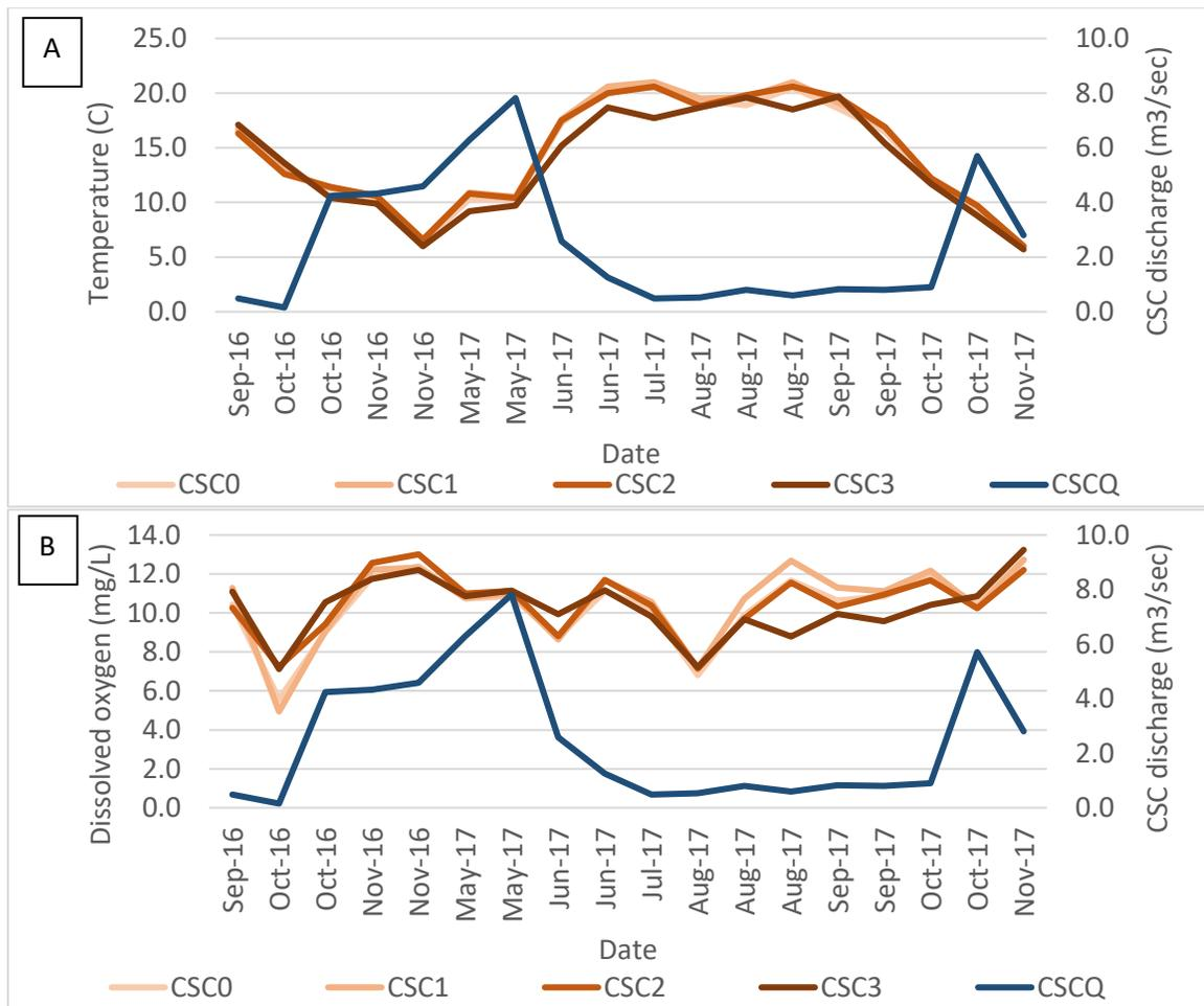
Figure 23. Water temperature (A) and dissolved oxygen (B) at connected side-channel sites (CSC) compared to connected side-channel discharge (CSCQ).
