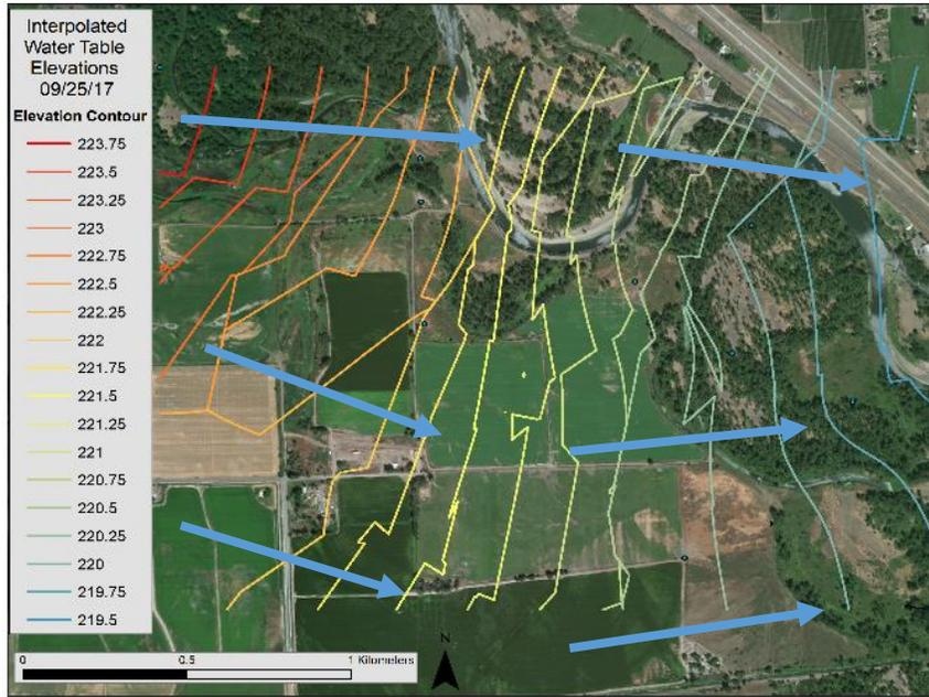
Figure 39. Water elevation contour lines interpolated from water level elevations using Empirical Bayesian Kriging in ArcMap 10.5. Blue lines indicate general direction of groundwater flow for 09/25/2017.
