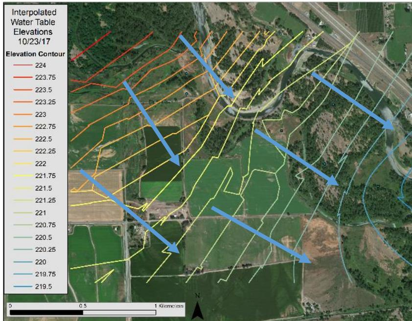
Figure 40. Water elevation contour lines interpolated from water level elevations using Empirical Bayesian Kriging in ArcMap 10.5. Blue lines indicate general direction of groundwater flow on 10/23/2017.
