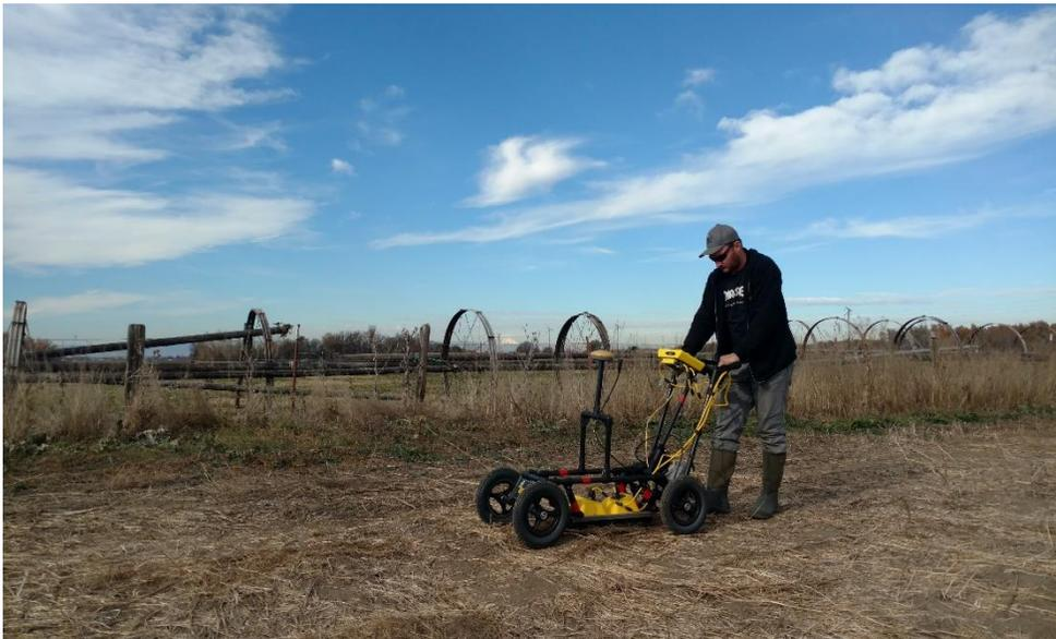
Figure 11. Sensors and Software GPR SmartCart setup with 500 MHz transducers recording readings at Well 13.
