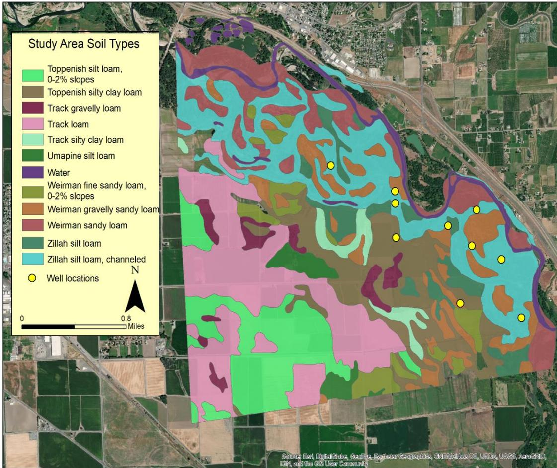
Figure 5. NRCS soil type definitions in the study area and locations of monitoring wells. Data from ESRI et al., Soil Data Viewer, ArcMap.
