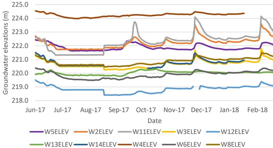
Figure 36. Groundwater elevations calculated from water table depths at 10 observation wells. Gaps in data lines indicate sensors not recording, flat portions indicate water levels below sensors.
