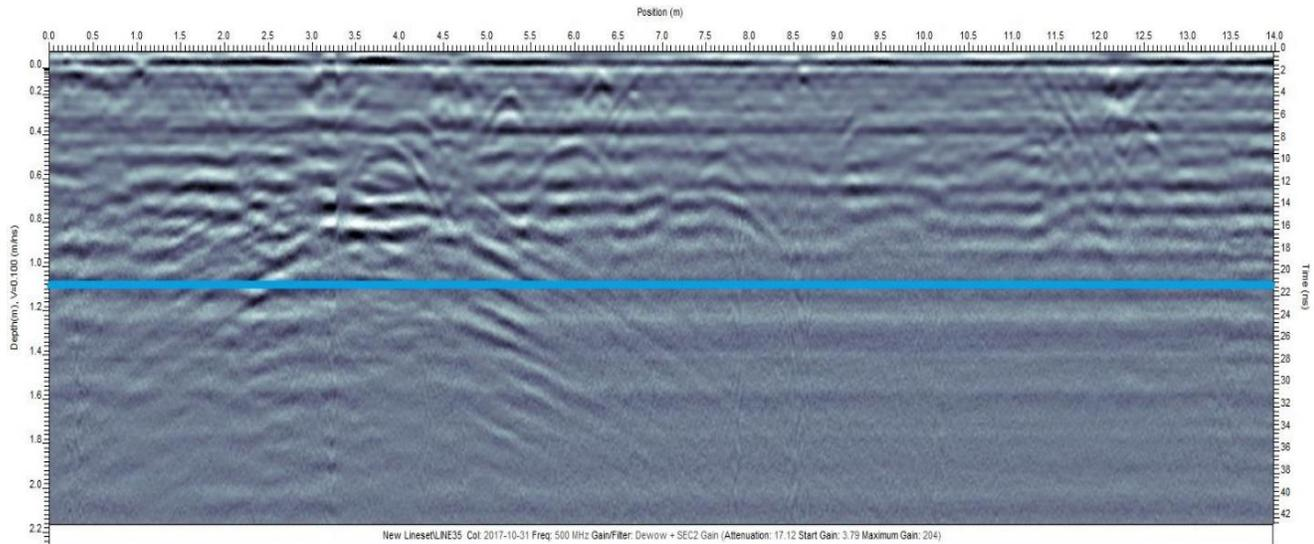
Figure 46. Radargram of the GPR transect at Well 12. The blue line represents the measured average daily water table depth.
