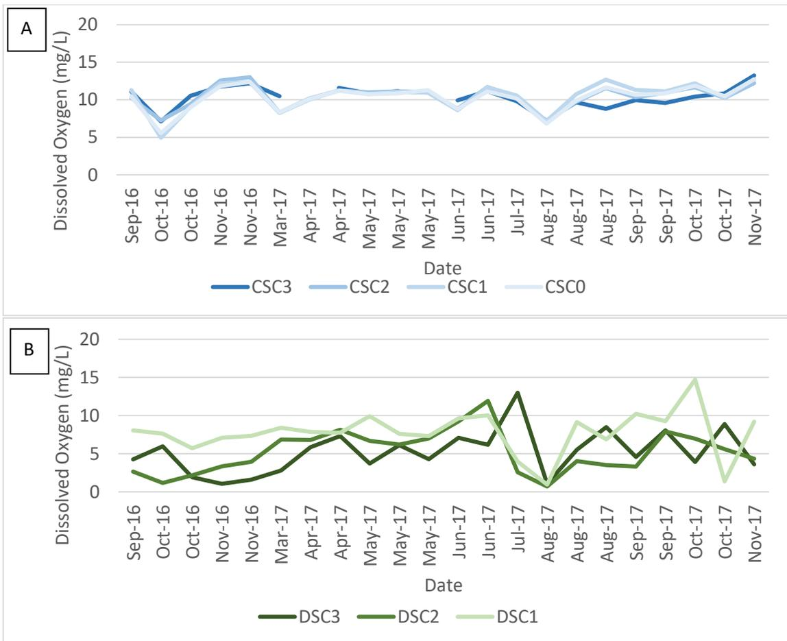
Figure 21. Comparisons of dissolved oxygen (mg/L) at connected side-channel (CSC) (A) and disconnected side-channel (DSC) (B) sites over the study period.
