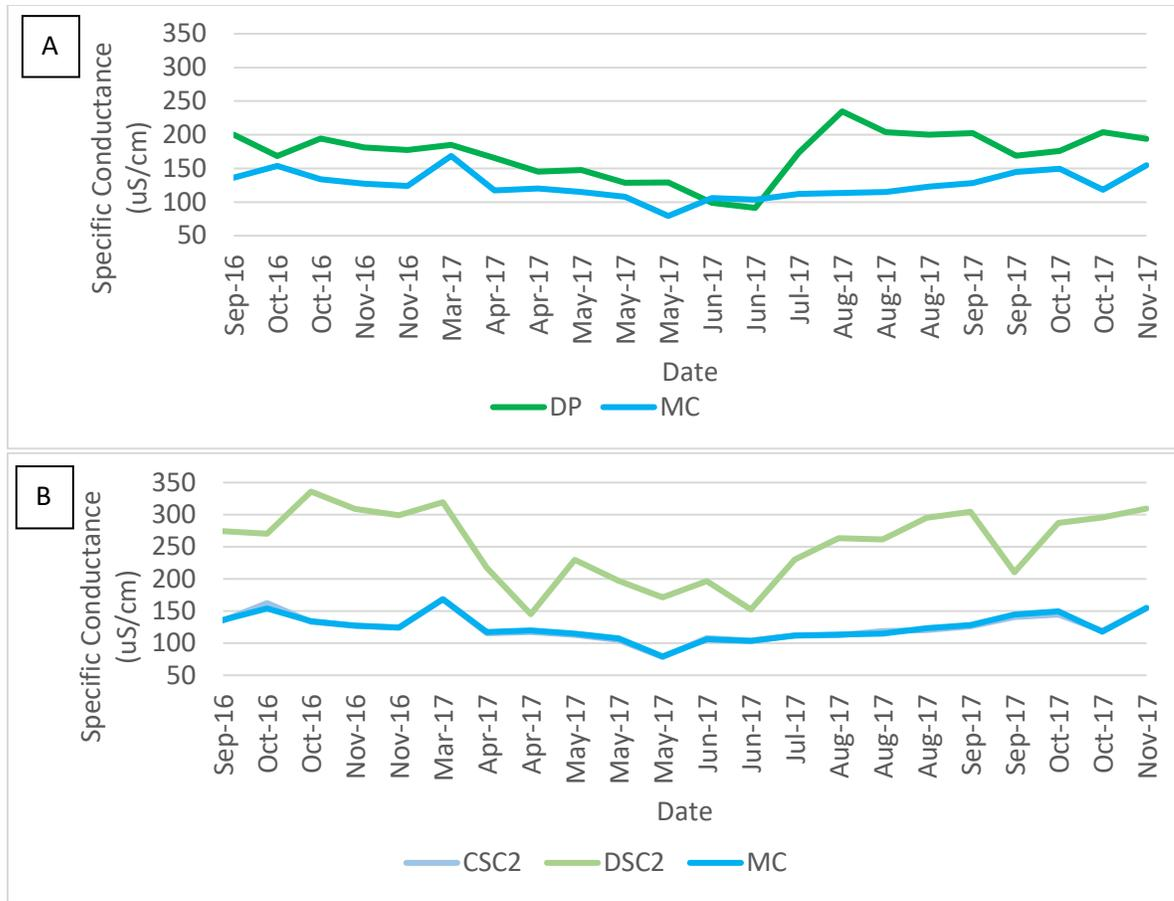
Figure 18. Comparisons of specific conductance (uS/cm) at sites over the study period at disconnected pond (DP) vs. main channel Yakima (MC) (A), and connected side-channel (CSC2), disconnected side-channel (DSC2) and main channel Yakima (MC) (B).
