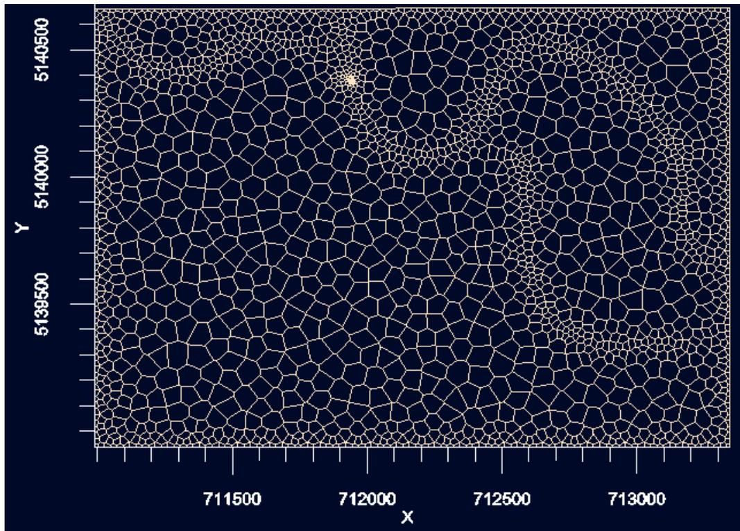
Figure 14. Unstructured V-grid created individual cells in Visual MODFLOW Flex. Cells are more dense around side-channels to increase the resolution of interactions around them.
