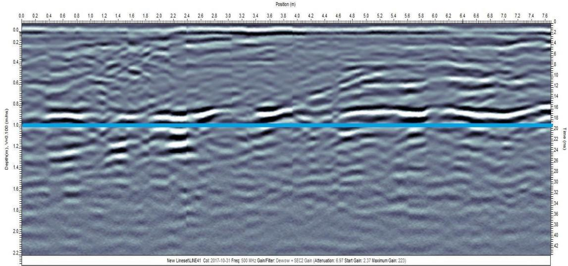
Figure 45. Radargram of the GPR transect at Well 5. The blue line represents the measured average daily water table depth.
