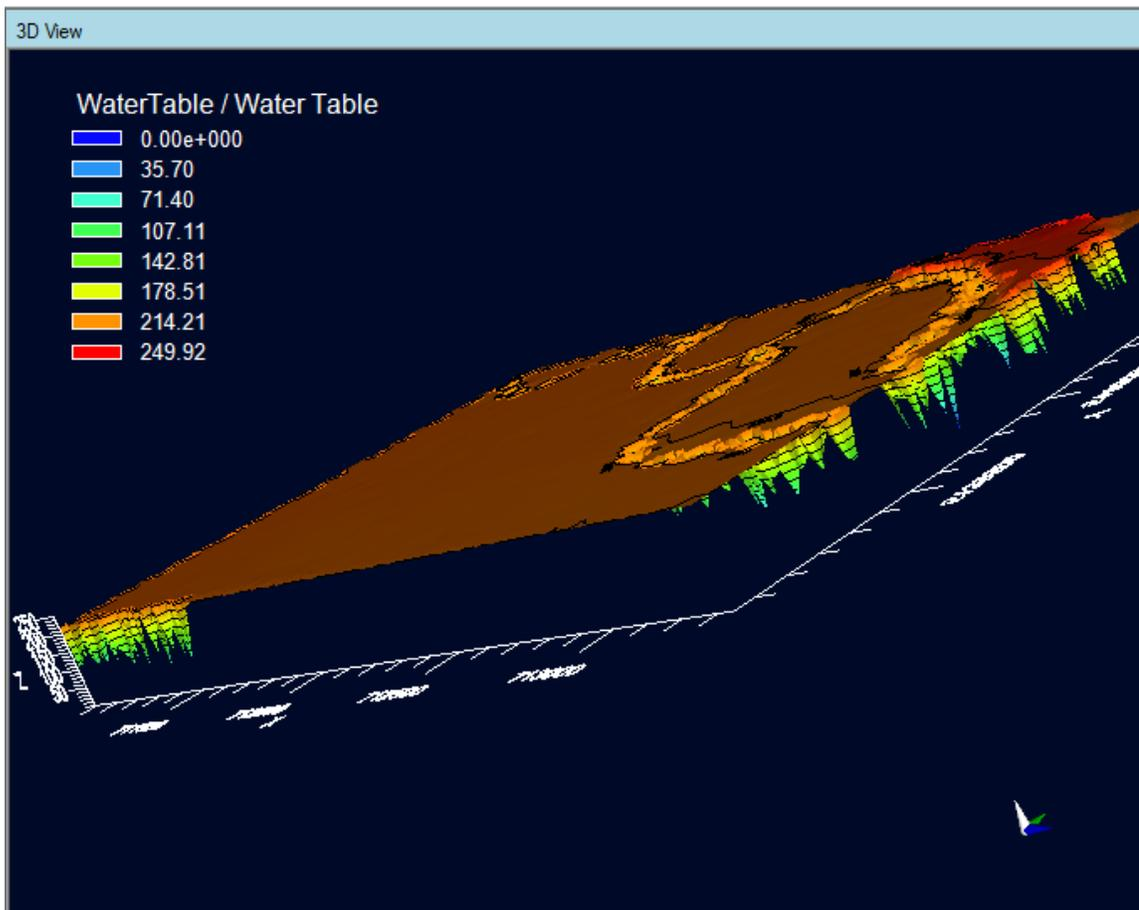
Figure 37. Unrealistic modeling result with the water table spiking below river features. The spikes mean that the software thinks the water table drops to an elevation of 0.
