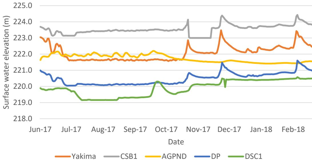
Figure 35. Surface water elevations calculated from water depths at four stage recorder sites and the Yakima River gage near Parker. Flat portions indicate water levels below sensor.
