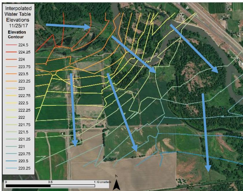
Figure 41. Water elevation contour lines interpolated from water level elevations using Empirical Bayesian Kriging in ArcMap 10.5. Blue lines indicate general direction of groundwater flow on 11/25/17.
