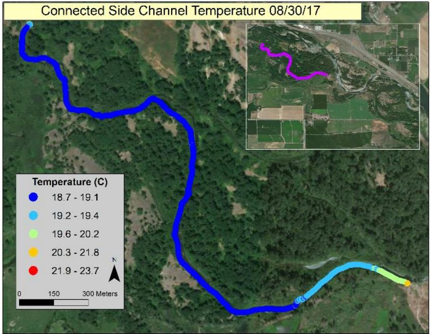
Figure 29. Connected side-channel temperature profiles for late summer.
