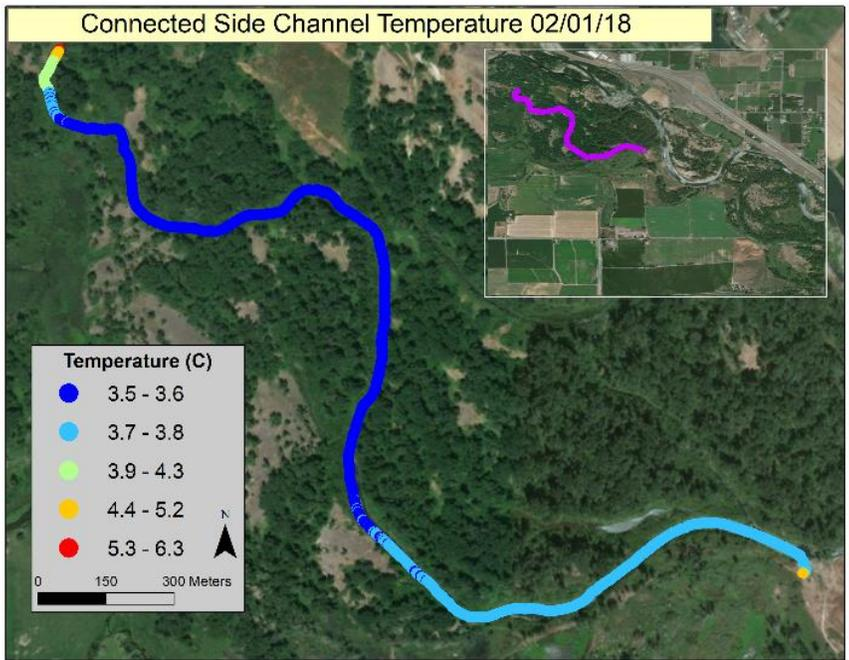
Figure 30. Connected side-channel temperature profiles for late winter.
