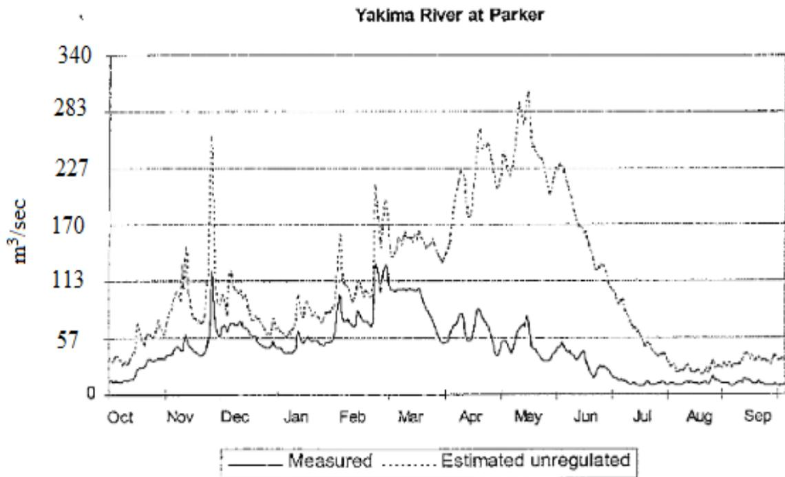
Figure 2. Hydrograph illustrating differences between the historic (unregulated) discharge of the Yakima River, versus the modern dammed and diverted river discharge at a USGS gauge at Parker, Washington, north of Meninick Wildlife Area. (Adapted from Tuck et al. 1999 p. 2-10).
