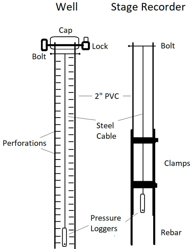
Figure 9. Diagrams of monitoring well and stage recorder designs. Not to scale.
