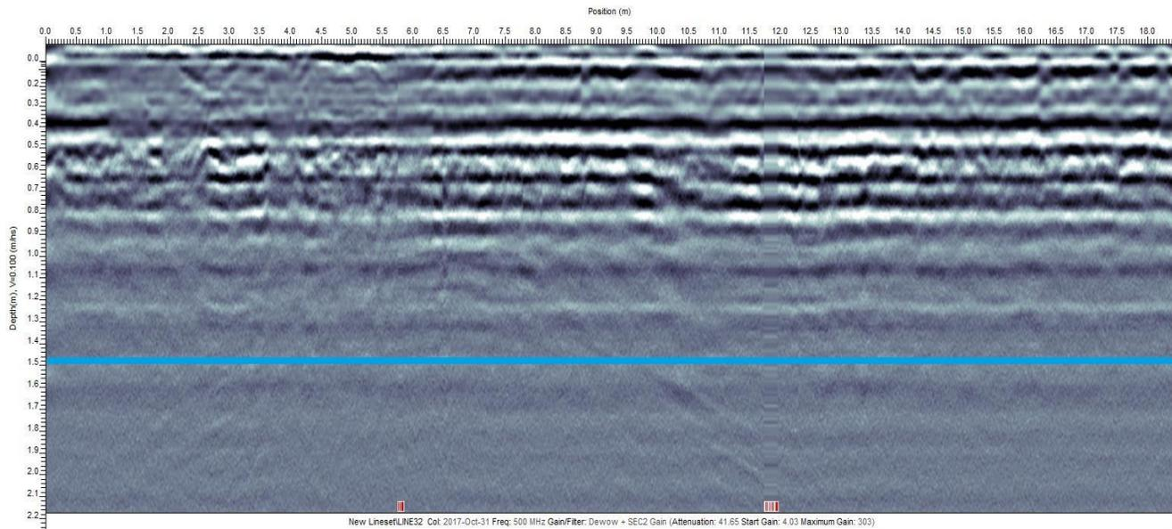
Figure 47. Radargram of the GPR transect at Well 13. The blue line represents the measured average daily water table depth.
