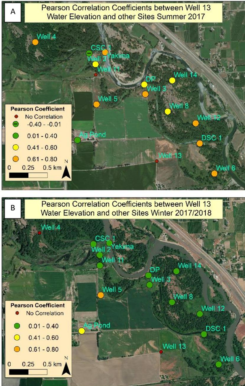
Figure 43. Pearson correlation coefficients between Well 13 water elevations and other water elevation sites in summer (A), and winter (B).
