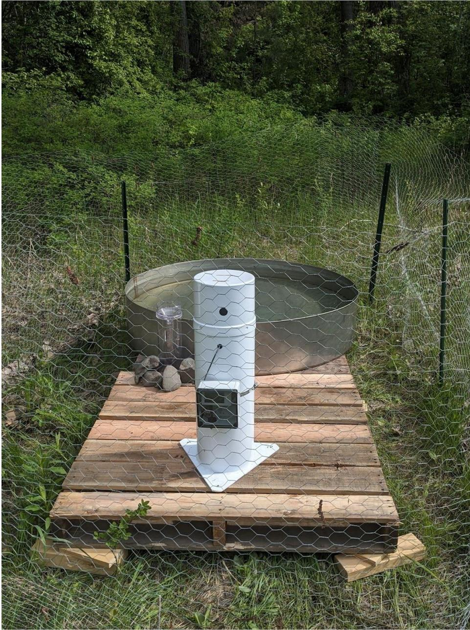
**Figure 11.** Photograph of evaporation station next to soil monitoring “riparian” site. The station is surrounded by 4 ft tall chicken wire fencing to discourage larger animals from drinking from the pan. The tall white cylinder is the evaporation gauge, which is directly connected to the pan and records its water level. A precipitation gauge seen next to the pan (transparent) was also deployed here.
